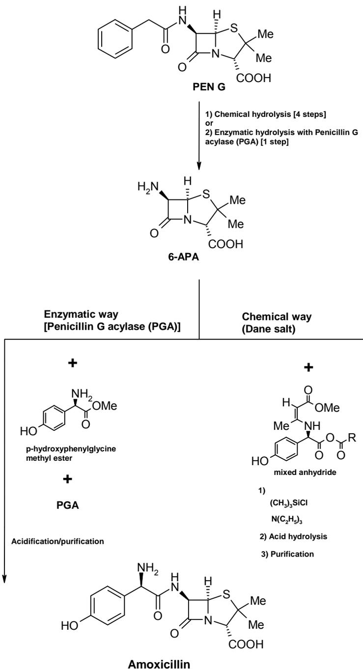
The conventional methods for chemically obtaining (using Dane salt) amoxicillin typically involve more than 10 steps, require low-reaction temperatures ( $-30^\circ\text{C}$ ), and use toxic solvents like methylene chloride and silylation reagents. It is reported that the production of one kilogram of amoxicillin generates up to about 70 kg of non-recyclable waste<sup>7</sup>.
